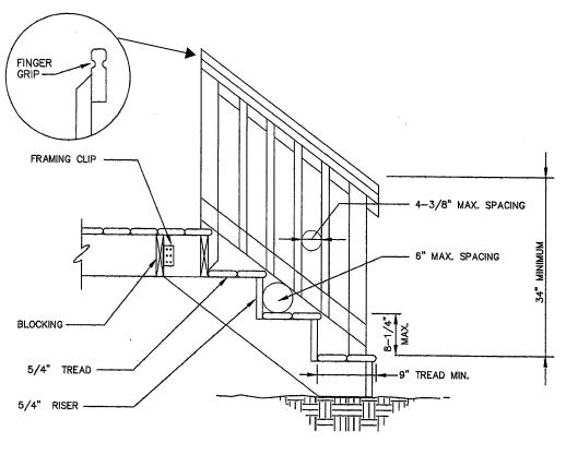
(311.7.1) STAIR WIDTH: STAIRWAYS SHALL BE NOT LESS THAN 36 INCHES IN CLEAR WIDTH AT ALL POINTS ABOVE THE PERMITTED HANDRAIL HEIGHT AND BELOW THE REQUIRED HEADROOM HEIGHT. THE CLEAR WIDTH OF STAIRWAYS AT AND BELOW THE HANDRAIL HEIGHT, INCLUDING TREADS AND LANDINGS, SHALL BE NOT LESS THAN 31-1/2 INCHES WHERE A HANDRAIL IS INSTALLED ON ONE SIDE AND 27 INCHES WHERE HANDRAILS ARE INSTALLED ON BOTH SIDES.
